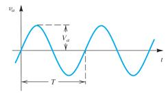
**FIG 5.** Sine-wave voltage signal of amplitude  $V_a$  and frequency f=1/T Hz. Angular frequency  $\omega=2\pi f$  rad/s
