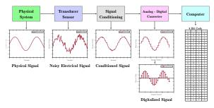
FIG 9. Digital data acquisition system<sup>1</sup>
