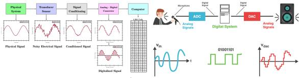
FIG 9. Digital data acquisition system<sup>1</sup>
