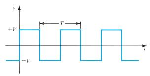
FIG 6. A square-wave signal of amplitude V
